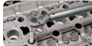
• Step 1 : Set up the torque value by torque wrench
