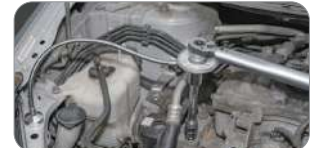
• Step 2 : Adjust the angle by angle gauge
